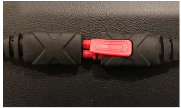
Figure 19 INCORRECT Insertion of Charger Plug
