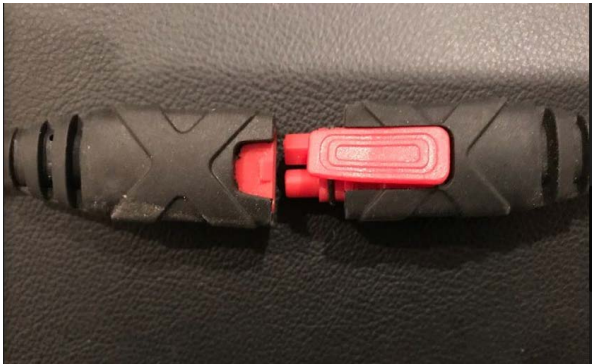
Figure 18 CORRECT Insertion of Charger Plug
